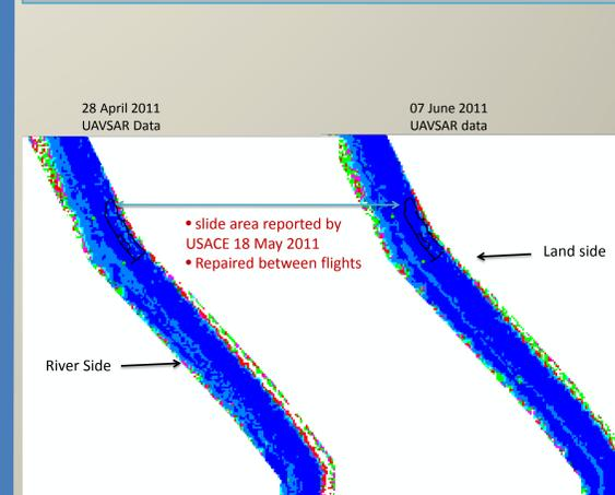
A new slide and seepage area on the land side of the levee was reported by USACE on 16 May 2011 during rising flood waters. The polygon shows the slide using coordinates taken during our field trip to this area. The 28 April 2011 classification result shows a unique class in this land slide, even before USACE reported discovering it. The slide might have occurred by 28, April 2011 or the H- alpha classification might be predicting the slide before it actually formed as an active slide.
