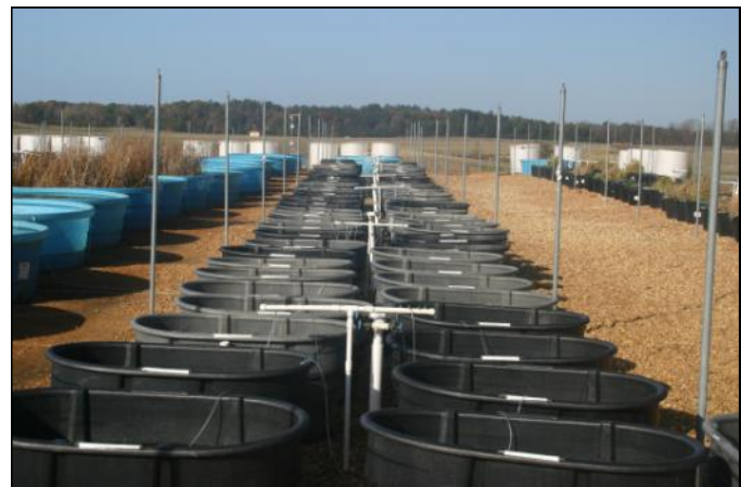
Figure 3. The mesocosm facility employs a wide range of tank sizes, from 50 to 500 gallons.
