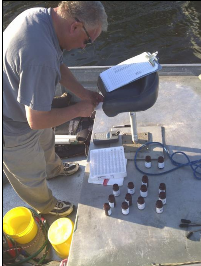
John Skogerboe, US Army Engineer Research and Development Center, analyzes water sample for Rhodamine WT as part of a herbicide dissipation study on Big Detroit Lake, MN, which is one of the collaborative efforts on invasive species management in which GRI was engaged in 2011.
