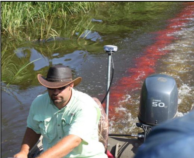
Ryan Wersal applying Rhodamine WT in the Ross Barnett reservoir, as part of a dissipation study for the Pearl River Valley Water Supply District. Rhodamine dye is used to examine how quickly water diffuses from a given location, which assists in selecting an herbicide, formulation, concentration, and application approach for control of invasive aquatic plants.
