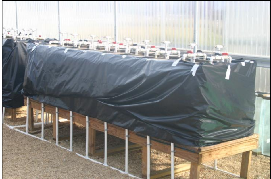
Figure 1. Thirty-six 30-gallon aquaria are used for small scale experiments in the aquatic plant greenhouse.
