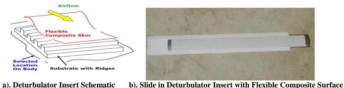
Figure 1. Structure of the FCSD Deturbulator
