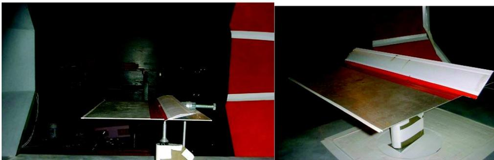
Figure 2. Deturbulator Test Model in Wind Tunnel
