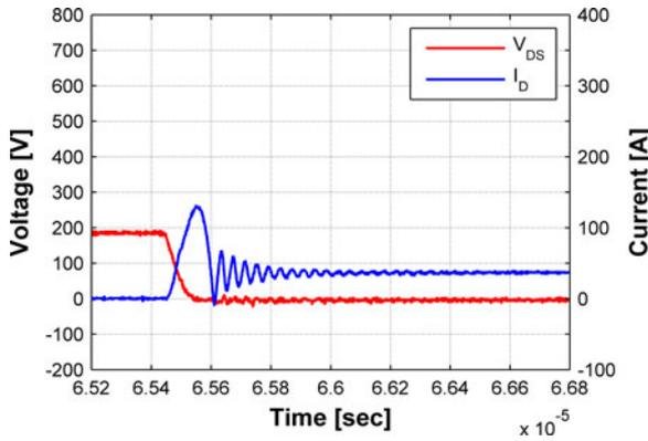
Fig. 3. Half-bridge turn-on showing shoot-through.
