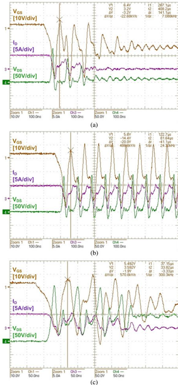
Fig. 11. Exemplary experimental waveforms corresponding to the histogram shown in Fig. 10. Subplots (a) and (c) demonstrate the occurrence of limited oscillation at  $V_{DS}/V_{CRIT}$  values of 0.33 and 3.0, respectively. Subplot (b) demonstrates the occurrence of sustained oscillation at a  $V_{DS}/V_{CRIT}$  value of 0.83.
