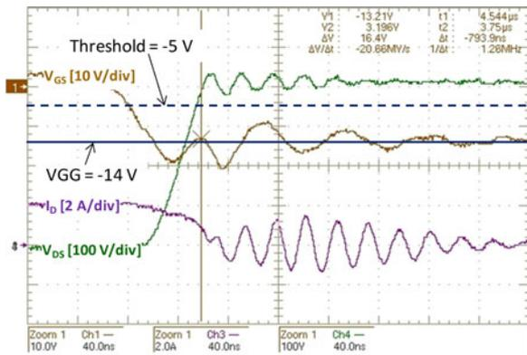
Fig. 9. No forced oscillation at  $V_{BUS} = 400$  V.
