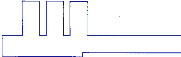
The physical boundary segment on which a single curvilinear coordinate is constant can have slope discontinuities, however, so that the L-shaped region above could have been considered to be composed of four segments instead of six, so that the transformed region becomes a simple rectangle:
