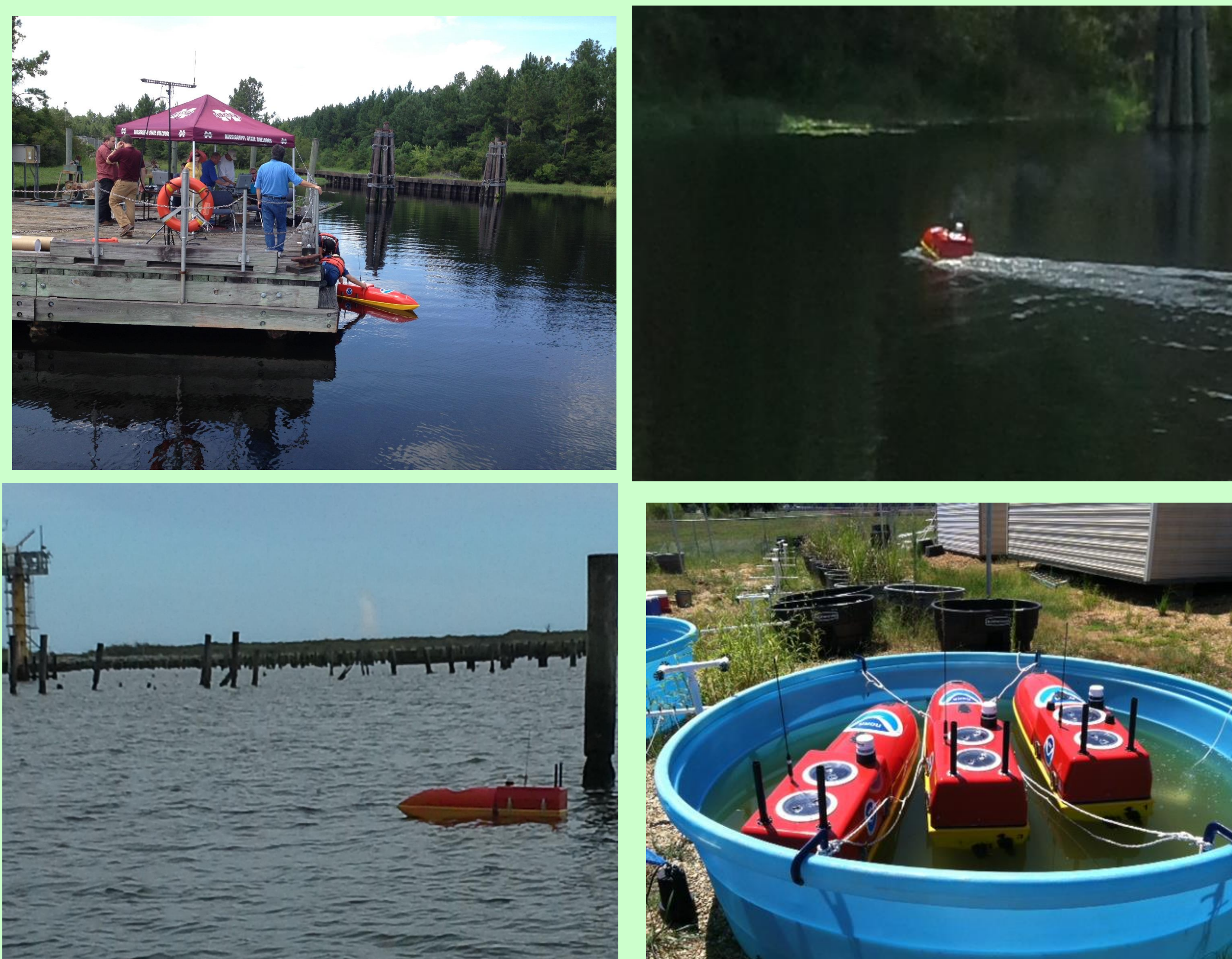
Figure 6. (Top) EMILY training exercise for MSU and NOAA personnel at Stennis Space Center's National Data Buoy Center canal, showing radio communication system and deployment (left), and an EMILY under propulsion (right). (Bottom) EMILY loitering near CMAN SHBL1 at Shell Beach, LA (left), and EMILYs undergoing tests in water tank at MSU (right).
