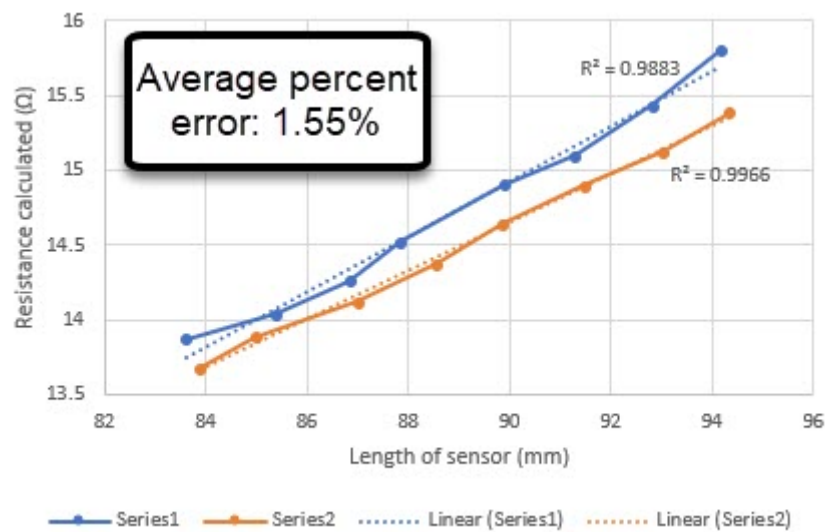
Figure 9. Comparison of Computing Unit and Micro-Ohm meter measurements collected.
