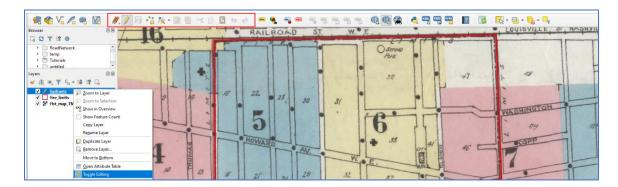
F. Click on the *Add Points Feature* button Hover the mouse cursor over the map and note that the cursor changed shape from an arrow to a scope-style symbol. This means that you are ready to add point features to the *hydrants* layer.
