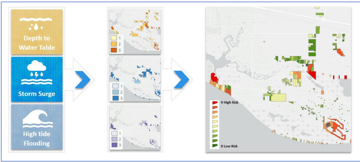
Figure 7. Collect and organize raster input layers; assign the vulnerability values; summarize parcels by vulnerability values from all input layers.
