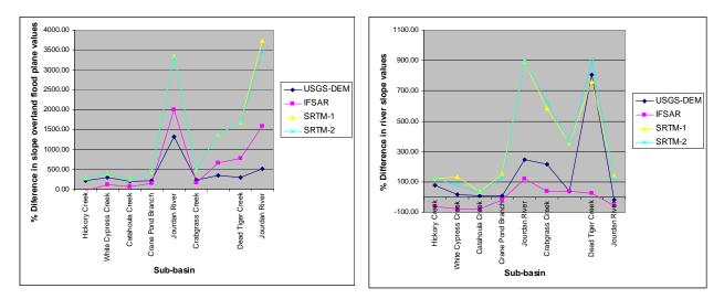
Figure 7. Percent differences for slope values (flood plane and river) with respect to NED-calculated values.
