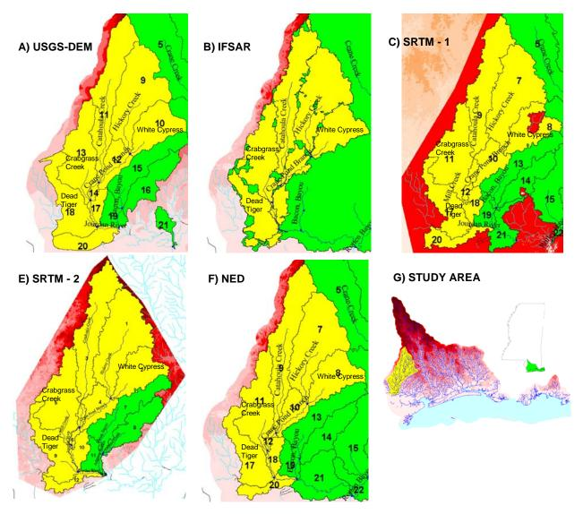
Figure 5. Watershed delineation using several elevation databases. Although the general distribution of sub-basins is similar, drainage areas for each sub-basin are different.
