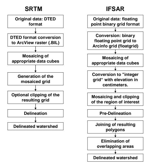
Figure 3. Methodology for watershed delineation using SRTM and IFSAR data.
