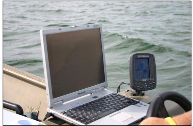
Fig. 2. Point intercept survey applications are run on a ruggedized computer for easy data entry on boats. A GPS antenna is on a pole at the back of the boat.
