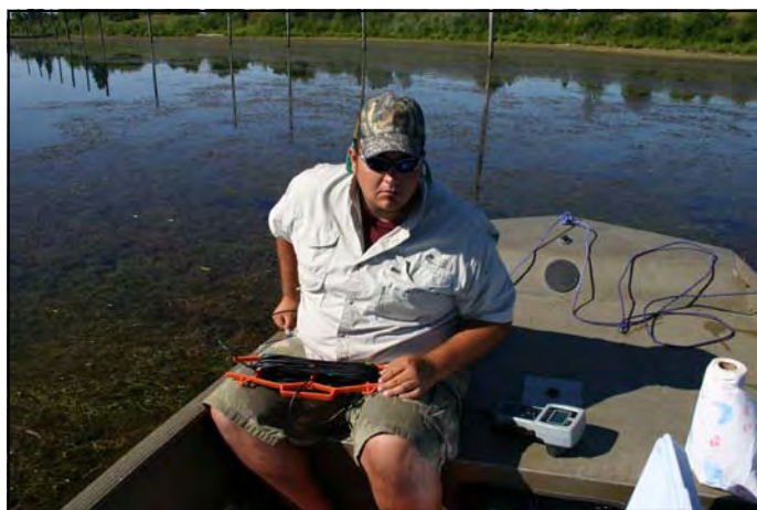
Photo 3. Waldemar Robles measures dissolved oxygen and temperature within a dense bed of vegetation on the Pend Oreille River near Cusick, WA.
