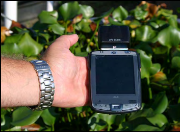
Fig. 1. Point intercept applications can be run on a handheld computer with a GPS antenna, for portability for both aquatic and terrestrial studies.
