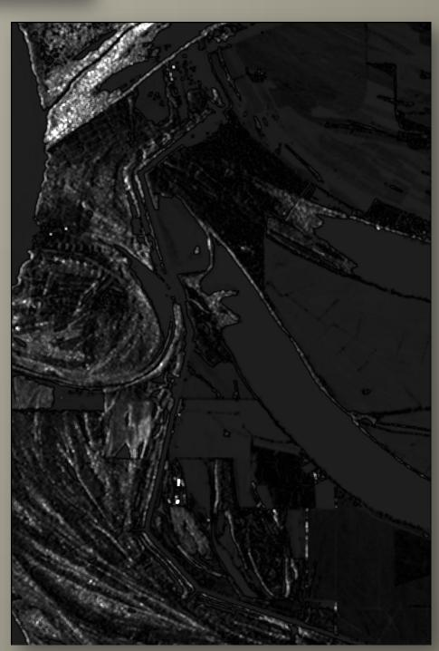
Statistical distance image between sand boil pixels and others in **AOI for Gray Level Co-occurrence Matrix features:** (R.) Window mean in HH (L.) homogeneity in HV;
