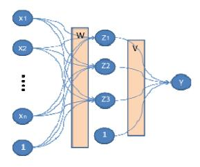
Figure 6. Backpropagation neural network with one hidden layer
