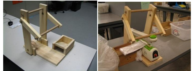
Figure 4. Lever System with Redesigned Platform
