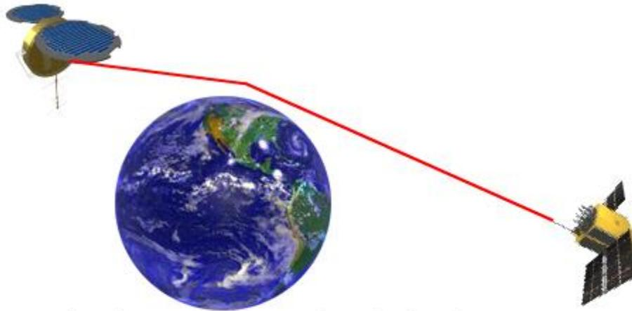
Transmitter satellite in higher orbit sends signals, which are received by LEO
