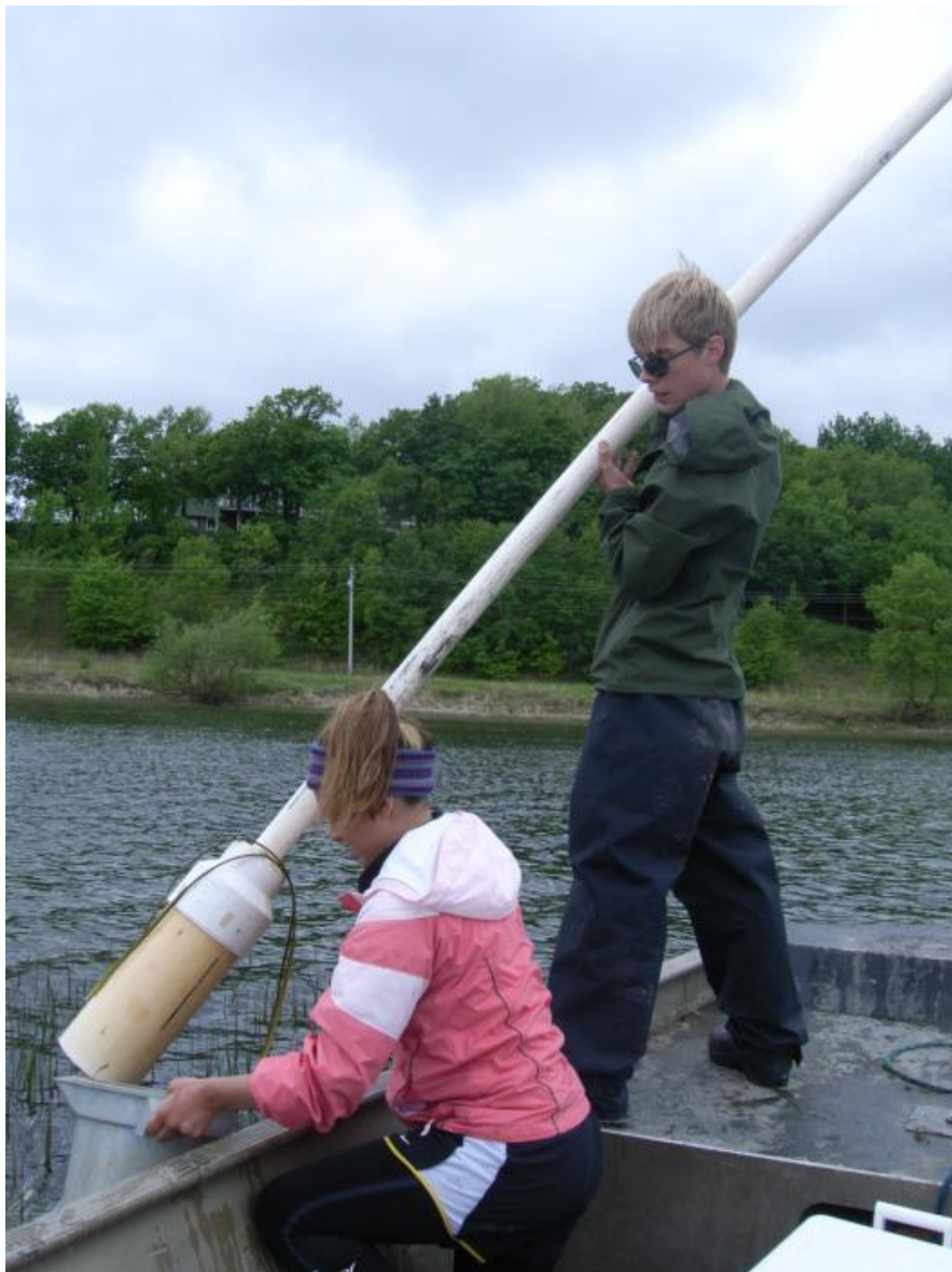
Figure 4. The 6" diameter coring device used to collect aboveground and belowground biomass of flowering rush in the Detroit Lakes.
