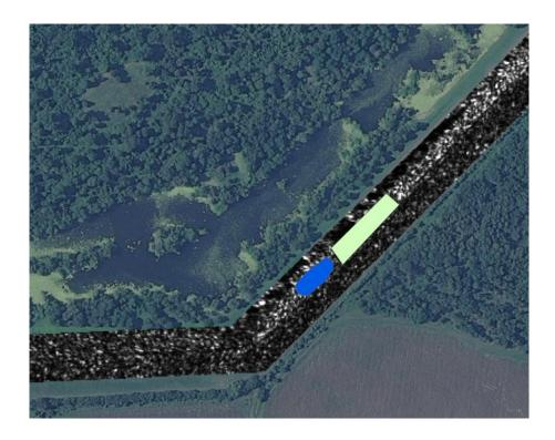
Fig. 4. TerraSAR-X radar data (HH polarization) overlaid with masks of slide (blue) and no-slide (green)
