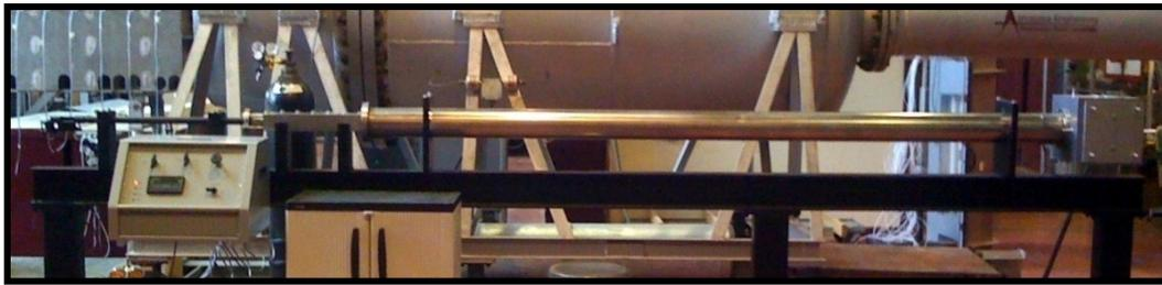
Figure 5. Mississippi State University micro two-stage light gas
