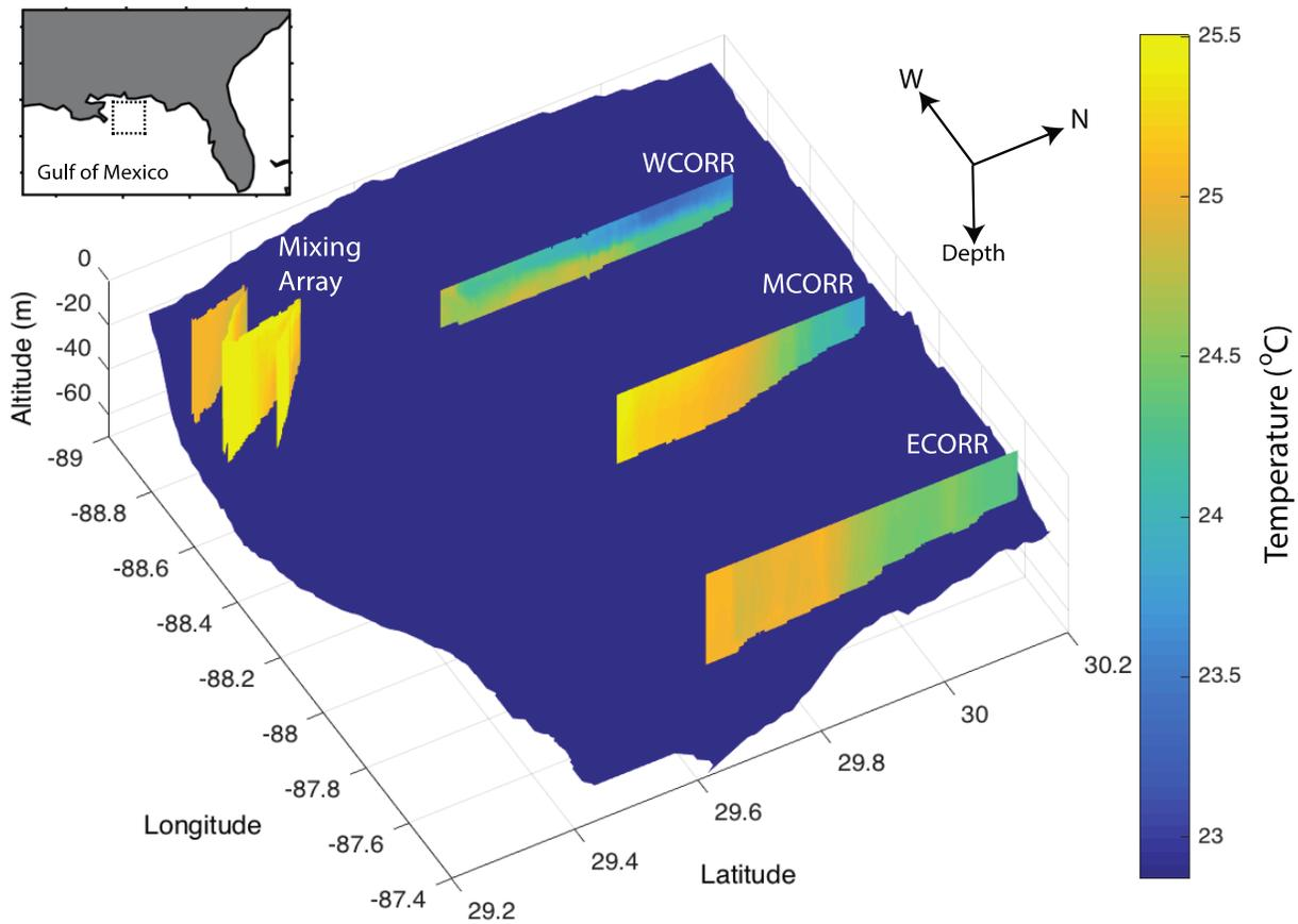
Temperature measured along 3 corridors with the In Situ Ichthyoplankton Imaging System (ISIS) (CTD attached to plankton imager)
