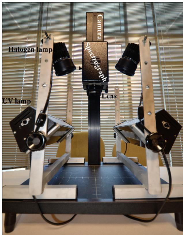
Figure 1. Hyperspectral imaging system.
