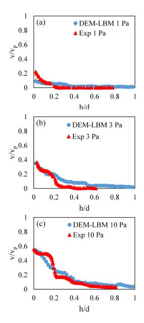
Figure 8. Comparison of shear profiles at applied stress levels of a) 1 Pa, b) 3 Pa, and c) 10 Pa. The particle velocity, v, was normalized by the plate velocity,  $v_p$ , and the distance from the plate, 337 338 h, was normalized by the gap width, d. The experimental data is from [3].
