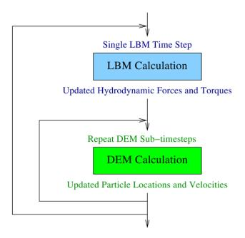
Figure 2. Diagram showing the sub-cycling process and updating of particle forces between the
