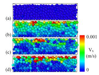
361 *Figure 10. Visualization showing the particles at time step of a) 0.0s, b) 0.5s, c) 0.75s, and d)* 1.5s for an applied stress of 10 Pa. The color corresponds to the particle velocity in the 362
