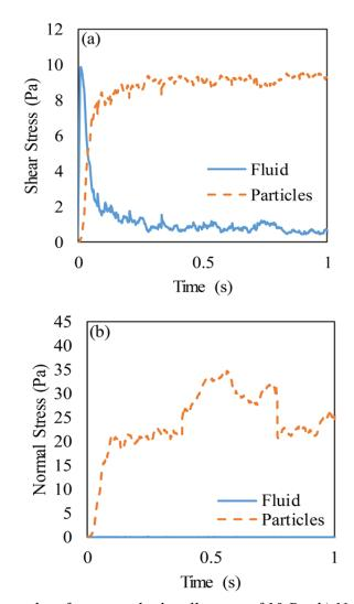
Figure 9. a) Shear stress plots for an applied wall stress of 10 Pa. b) Normal stress plots for an
