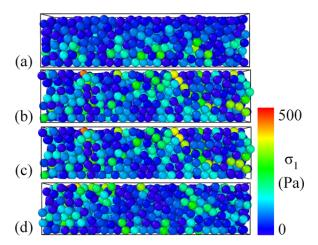
Figure 11. Visualization showing maximum compressive stress of each particle for a)0.0s b)0.5s 366 367 c)0.75s and d)1.5s. 368
