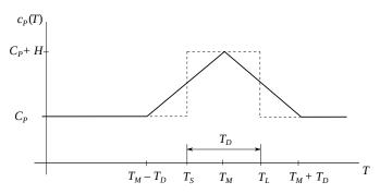
Figure 3: Representation of the latent heat.
