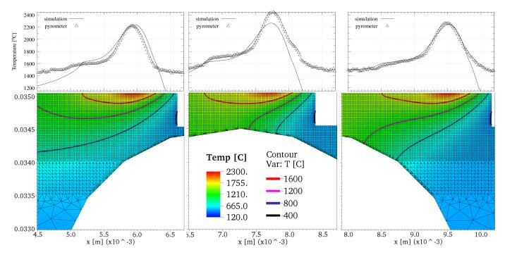
Figure 5: Comparison of simulation results with pyrometer data when depositing above largest void. Bottom-center subfigure is a magnified portion of Figure 4.
