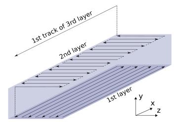
Figure 2: Deposition direction of successive layers.
